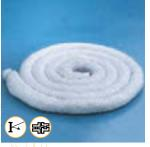
Flexible sleeve braided with glass fibres, treated high-temperature, reinforced with a yarn made of nickel-chrome alloy, around a core containing high-temperature carded glass fibres and natural fibres.
