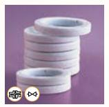
Packing consisting of a PTFE-impregnated plaited core made of carbon yarns, covered with a plaited sleeve of impregnated and lubricated PTFE yarns.
