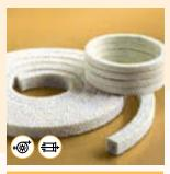
Packing made of special polyacrylic yarns. Each single yarn is impregnated with PTFE using our exclusive «Filcoat»-process. The packing is then re-impregnated during plaiting operation in a bath consisting of PTFE mixed with a food-quality silicone lubricant.
