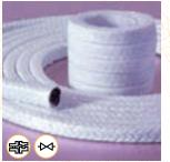
Packing consisting of a braided core made from PTFEimpregnated carbon yarns and a sleeve made from crossbraided, impregnated and lubricated PTFE yarns.
