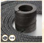
Packing made from high-purity expanded graphite yarns (>99.5%C) coated with inconel yarns, impregnated with a high-purity graphite mix (>99.5%C) and incorporating an additional agent to improve friction coefficient.
